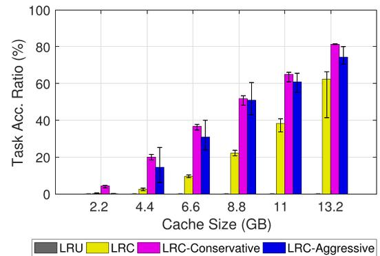
Fig. 15. Task acceleration ratio with different cache policies on a 50-node cluster.
