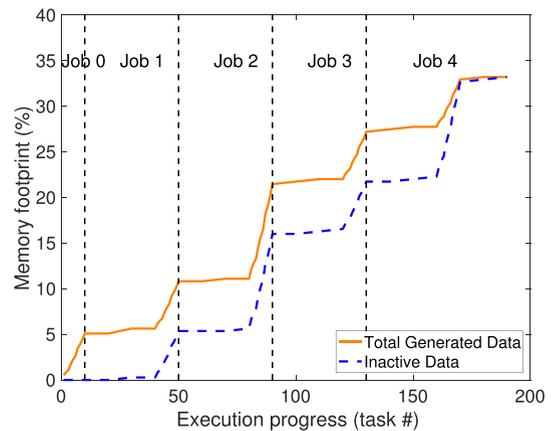
Fig. 3. Memory footprints of intermediate data generated and inactive blocks cached during the execution of *Connected Component*, an application in SparkBench [16].
