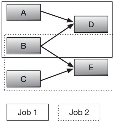
Fig. 8. An example DAG to illustrate the workflow of LRC-Online, where blocks  $D$  and  $E$  are respectively computed by Job 1 and Job 2. The former is submitted earlier than the latter.
