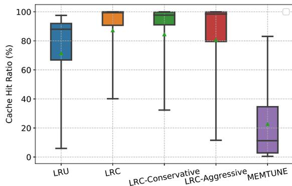
Fig. 21. Cache hit ratio under different cache policies with the Alibaba trace. Boxes show the 25th percentile, mean, and 75th percentile, and whiskers depict the 5th and 95th percentiles. Quantiles are the same in Figs. 22 and 23.
