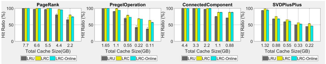
Fig. 17. Cache hit ratio under the three cache management policies with different cache sizes.
