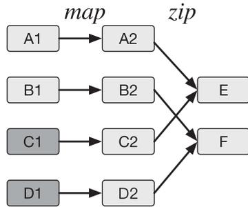
Fig. 1. The data dependency DAG of an example application. Each block represents a dataset. Two of the input blocks,  $A_1$  and  $B_1$ , are cached in memory, while the other two input blocks,  $C_1$  and  $D_1$ , are stored on disk. Blocks  $A_2$ ,  $B_2$ ,  $C_2$ , and  $D_2$  are intermediate datasets derived from each of the four input datasets via mapping. Block  $E$  ( $F$ ) is the final result derived from both  $A_2$  and  $B_2$  ( $B_2$  and  $D_2$ ).
