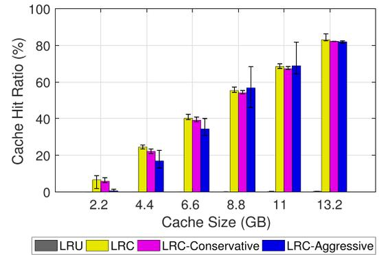
Fig. 14. Cache hit ratio with different cache policies on a 50-node cluster.
