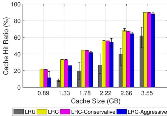
Fig. 11. Cache hit ratio with different cache policies on a 10-node cluster.
