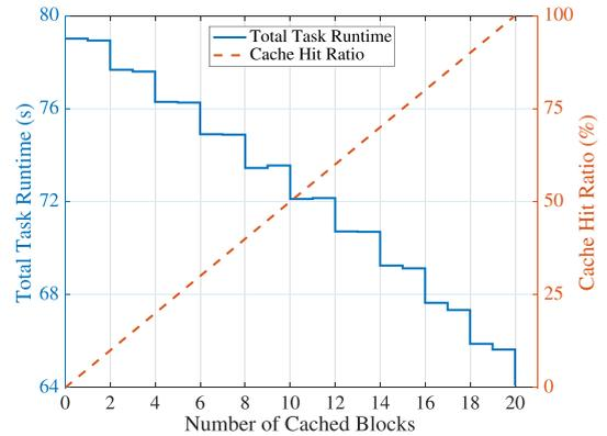
Fig. 6. Total task runtime of the example job in Fig. 5, with the cached RDD blocks increasing one at a time in the order of  $A_1, B_1, A_2, B_2, \dots, A_{10}, B_{10}$ .
