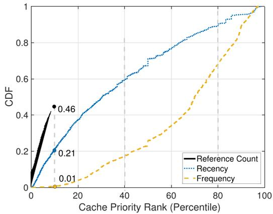
Fig. 7. Distribution of the cache priority ranks of accessed data blocks with respect to recency, frequency, and reference count. The workloads cover all SparkBench applications [16].
