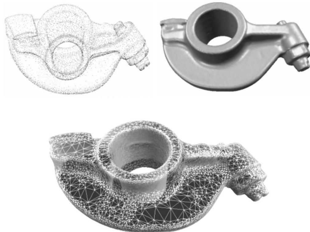
Fig. 10. Rocker arm. Top left: point cloud. Top right: reconstructed mesh surface. Bottom: the reconstructed mesh from non-regular point cloud.
