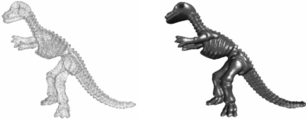
Fig. 5. Dragon. Left: point cloud. Right: reconstructed mesh surface.
