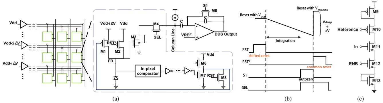
Fig. 5. (a) Diagram of circuit I with in-pixel comparator for auto-reset. (b) Principal of shifting at reset phase and circuit timing. (c) In-pixel comparator.
