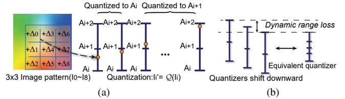
Fig. 1. The PSD algorithm (a) If there are more neighboring pixels quantized to  $A_{i+1}$ , then the pixel value in interval  $[A_i, A_{i+1}]$  is more closer to  $A_{i+1}$  other than  $A_i$ . (b) Quantizers shift downward when  $\Delta_i > 0$ . Multiple coarse quantizers for an image patch is equivalent to a single quantizer with high accuracy. DR loss occurs due to coarse quantization for bright pixels.
