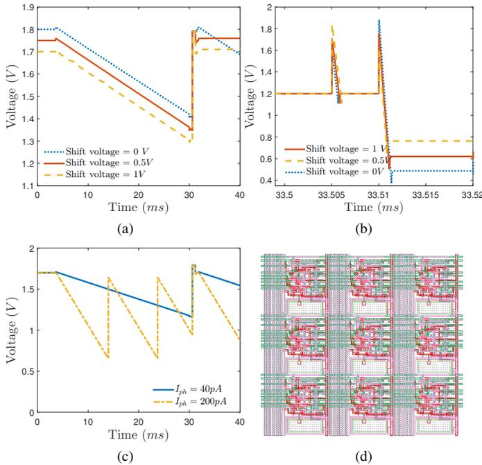
Fig. 6. (a) Shift at reset: there is a shift between two resets. (b) DDS output of circuit I: shifts are 0V, 0.5V and 1V respectively for pixels with the same values (c) Auto-reset (d) Pixel layout for circuit I with auto-reset
