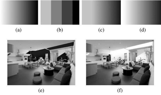
Fig. 3. Simulation result of auto-reset PSD. (a) Original image of gray scales. (b) Image quantized with 2 bits directly. (c) PSD reconstructs image with much improved quality, but there is noticeable DR loss for bright pixels. (d) Image reconstructed by auto-reset PSD is free of DR loss. (e) Modulo image for an indoor environment. (f) Reconstructed scene by auto-reset PSD using 2 bits.
