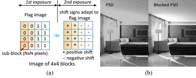
Fig. 2. (a) In blocked PSD, sign of shifts are adapted to the illumination for each sub-block. (b) Reconstruction image using PSD (left) and blocked PSD (right) using just 2 quantization bits.
