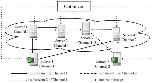
Fig. 1. A multi-source multi-channel overlay live streaming network with server collaboration.
