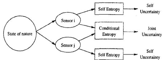
Figure 1: Modelling Sensor Interdependence
