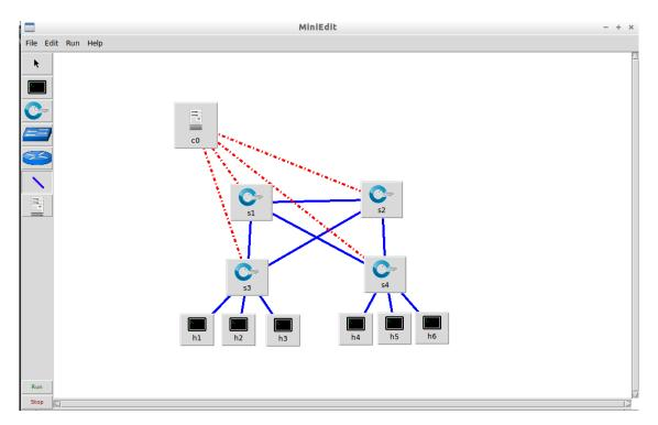
In a SDN network, control panel and data panel is separated. Due to such architecture, the control plane is centralized, so the controller recognizes entire network environment. The centralized controller thus can control the network's traffic flow in a bigger picture, and the controller can add/edit/remove entries of flow table in switches for traffic decision.
