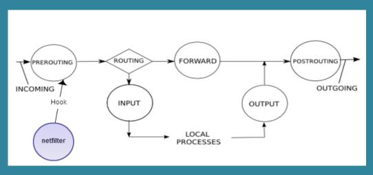
In the AP kernel, A Netfilter is added to hook the pre-routing stage and control the traffic according schedule.
