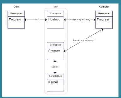
Client and AP are simply connected by Wifi, socket programming between AP and controller is the network communication tool,
