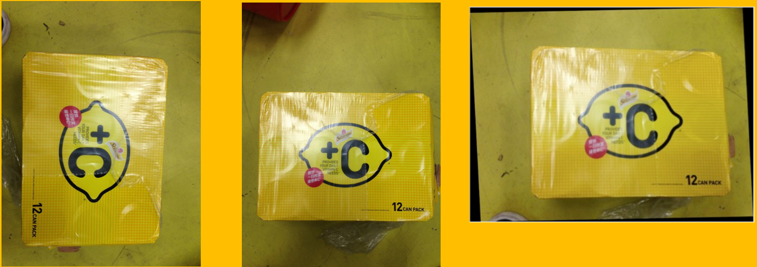
Figure 4. The first two images are photo taken of the same box from different angles. Using features matching and RANSAC we are able to apply transform to the first image to produce the third image, which transform the box to the same orientation as the second box.
