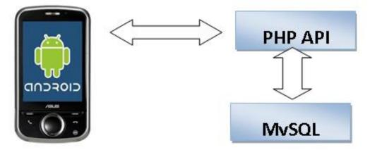
In short, if users try to search items from the application, an http request with parameters is sent to the PHP in JSON format. Then, the PHP decode the parameters and get the required data from the database. Then, it returns data back to the android device.
