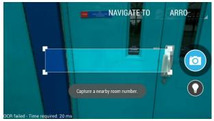
Figure 3. Phase I: OCR Room Number Input
