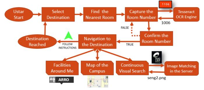
Figure 2. Ustar Run-Through Flow Chart
