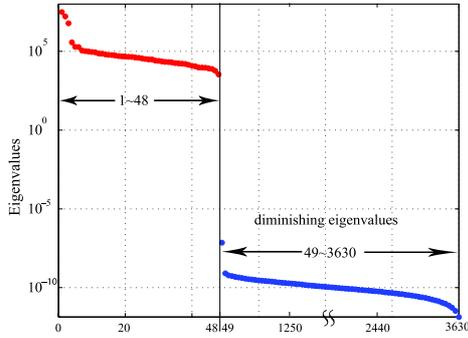
**Fig. 3.** Spectrum of a  $3630 \times 3630$  matrix  $\mathbf{Q}$ , computed from our experimental data, indicates that only the largest 48 eigenvalues are strictly positive, and the rest are insignificant. The spectrum clearly reflects the low-rank nature of the matrix  $\mathbf{Q}$  and the feasibility of low-rank approximation.
