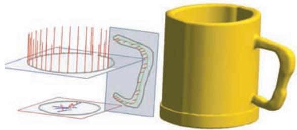
**Figure 12:** Cup shape. Skeleton structure and resulting surface.
