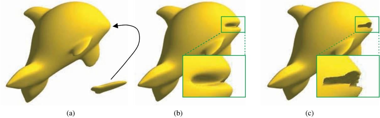
**Figure 10:** Carving vs. Boolean operation. (a) shows a whale shape and a carving tool. (b) and (c) are the results of soft carving and hard subtraction operation, respectively. All the whales are polygonalized at the same resolution.
