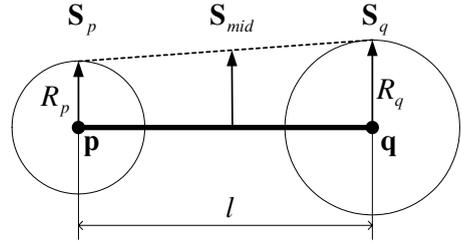
Figure 7: Convolution surface from a line segment.
