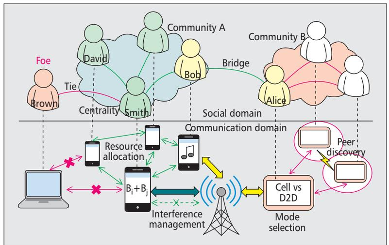
**Figure 1.** Illustration of social-aware D2D communication underlying cellular system, where in the communication domain devices gain access to the cellular BSs or establish D2D communication subject to the physical and communication constraints, while in the social domain devices form a mobile social network regulated by stable social relationships and phenomena.
