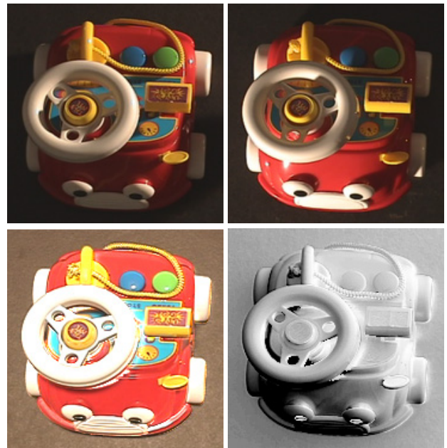
Figure 5: The top row shows two typical views of our noisy data, where shadows and highlight are present on the complex object. The bottom left shows the recovered albedo. The bottom right shows the recovered surface normals displayed using \mathbf{N} \cdot \mathbf{L} with \mathbf{L} = (\frac{1}{\sqrt{3}}, \frac{1}{\sqrt{3}}, \frac{1}{\sqrt{3}})^T . Please see supplementary video [1].
