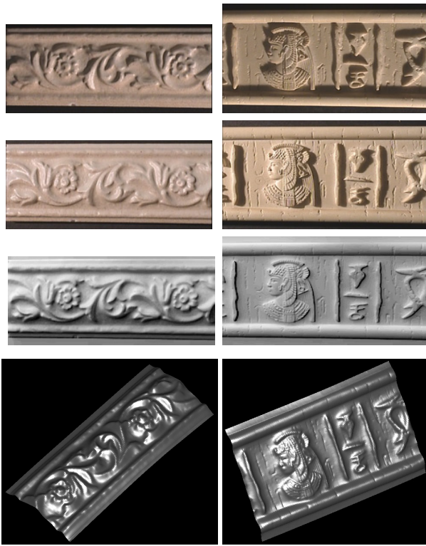
Figure 4: Results on two tiles. The top two rows show two typical images we captured. The reconstructed normals are shown here as \mathbf{N} \cdot \mathbf{L} with \mathbf{L} = (-\frac{1}{\sqrt{3}}, \frac{1}{\sqrt{3}}, \frac{1}{\sqrt{3}})^T . The last row shows the reconstructed surfaces at novel viewpoints.
