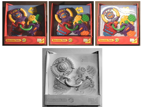
Figure 6: Three typical images for this object are shown in the top, where many assumptions in photometric stereo are violated: shadows, highlight, transparency, and inter-reflections due to the complex geometry and spatially-varying albedos. The recovered normals \mathbf{N} at each pixel, displayed here as \mathbf{N} \cdot \mathbf{L} with \mathbf{L} = (\frac{1}{\sqrt{3}}, \frac{1}{\sqrt{3}}, \frac{1}{\sqrt{3}})^T , are very reasonable.
