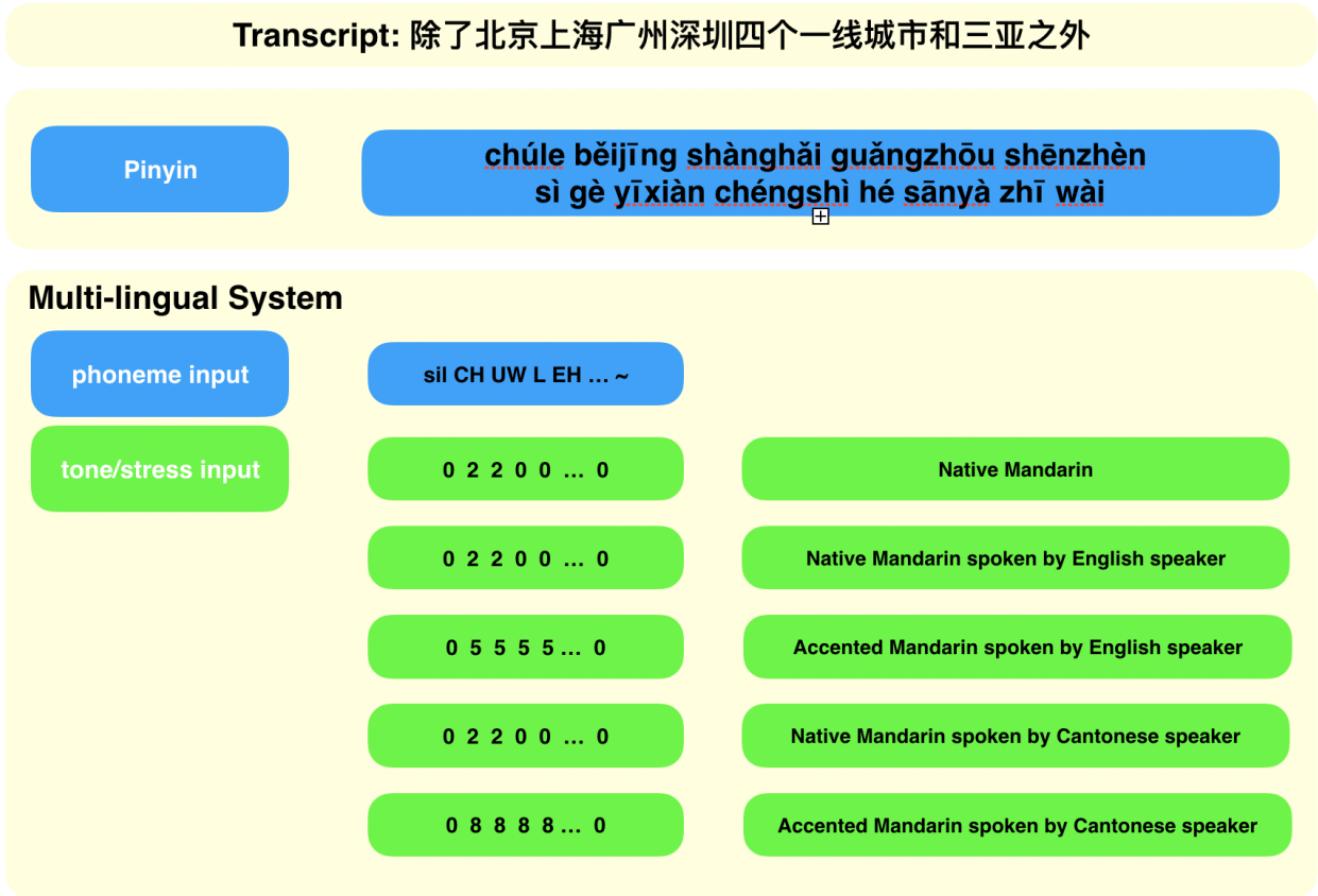
Figure 3.3: Linguistic feature inputs for synthesizing a Mandarin utterance in native Mandarin, Cantonese speakers’ native/accented Mandarin and English speakers’ native/accented Mandarin.
