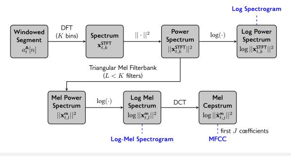
\* The flowchart shows the extraction of one frame of features given a windowed segment, and the blue texts give the terminologies corresponding to a feature sequence.
