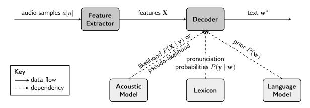
Figure 2.1: Schematic diagram of a typical modularized ASR system
