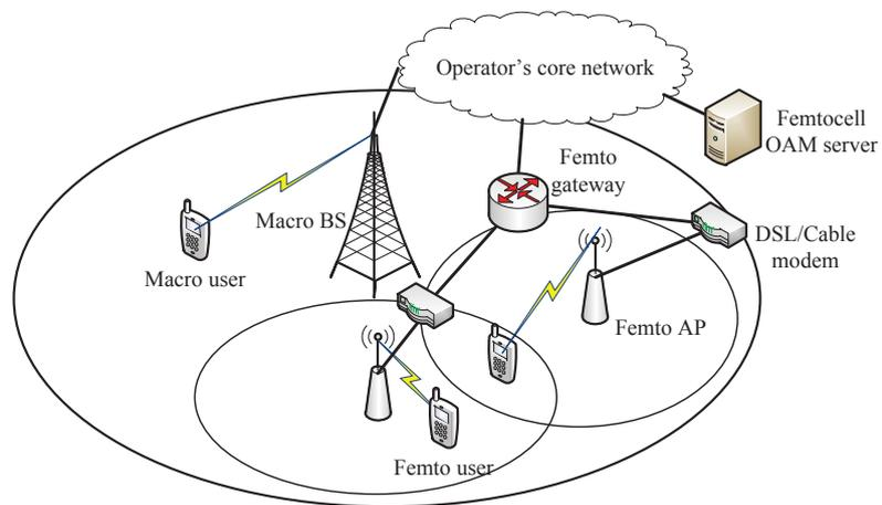
Fig. 1. Femtocell network architecture
