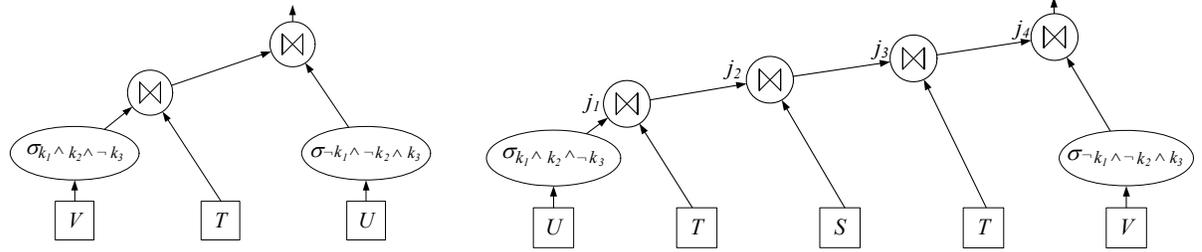
(a) Operator tree for  $(V\{k_1, k_2\}, T, U\{k_3\})$  (b) Operator tree for  $(U\{k_1, k_2\}, T, S, T, V\{k_2, k_3\})$
