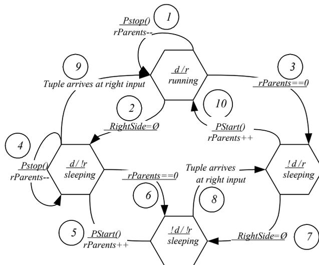
Fig. 27. States and transitions for join operators
