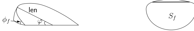
Figure 3: Left: The face f makes an angle \phi_f with the horizontal, and the ascent is \text{len} \cdot \sin \varphi \sin \phi_f . Right: The bold segment represents the clipping.
