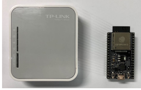
Fig. 5. The prototypes of sensors and tags in the experiment. The left one is the sensor running on TP-Link MR3020, and the right one is the tag implemented on the platform of Espressif ESP32.
