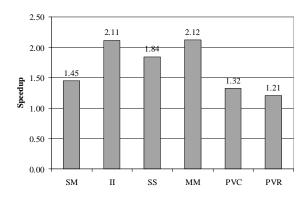
Figure 7: The performance speedup of coalesced accesses on the GPU.
