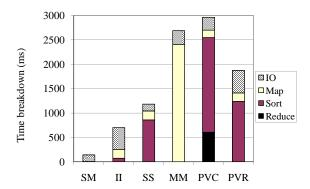
Figure 6: The time breakdown of Mars on the six applications with the large data set.
