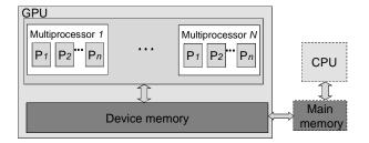
Figure 1: The many-core architecture of GPU.
