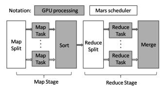
Figure 2: The work flow of Mars on the GPU.
