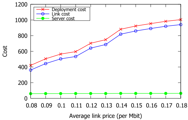
Fig. 10. Components of deployment cost versus average link price for CO-COS.
